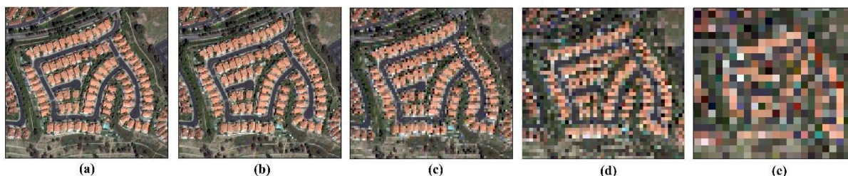
Figure 2. Comparison of varying spatial resolution: a) 0.5 m, b) 2m, c) 4m, d) 8m, e) 16m
